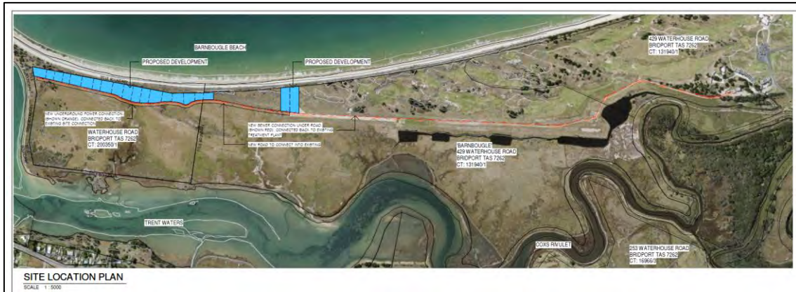
Figure 15 – Revised Site Plan Ap01 Rev 005, dated 23/06/23, showing an underground power connection heading east towards the existing electrical infrastructure at Barnbougle Dunes (source: 6ty Degrees 2023).
