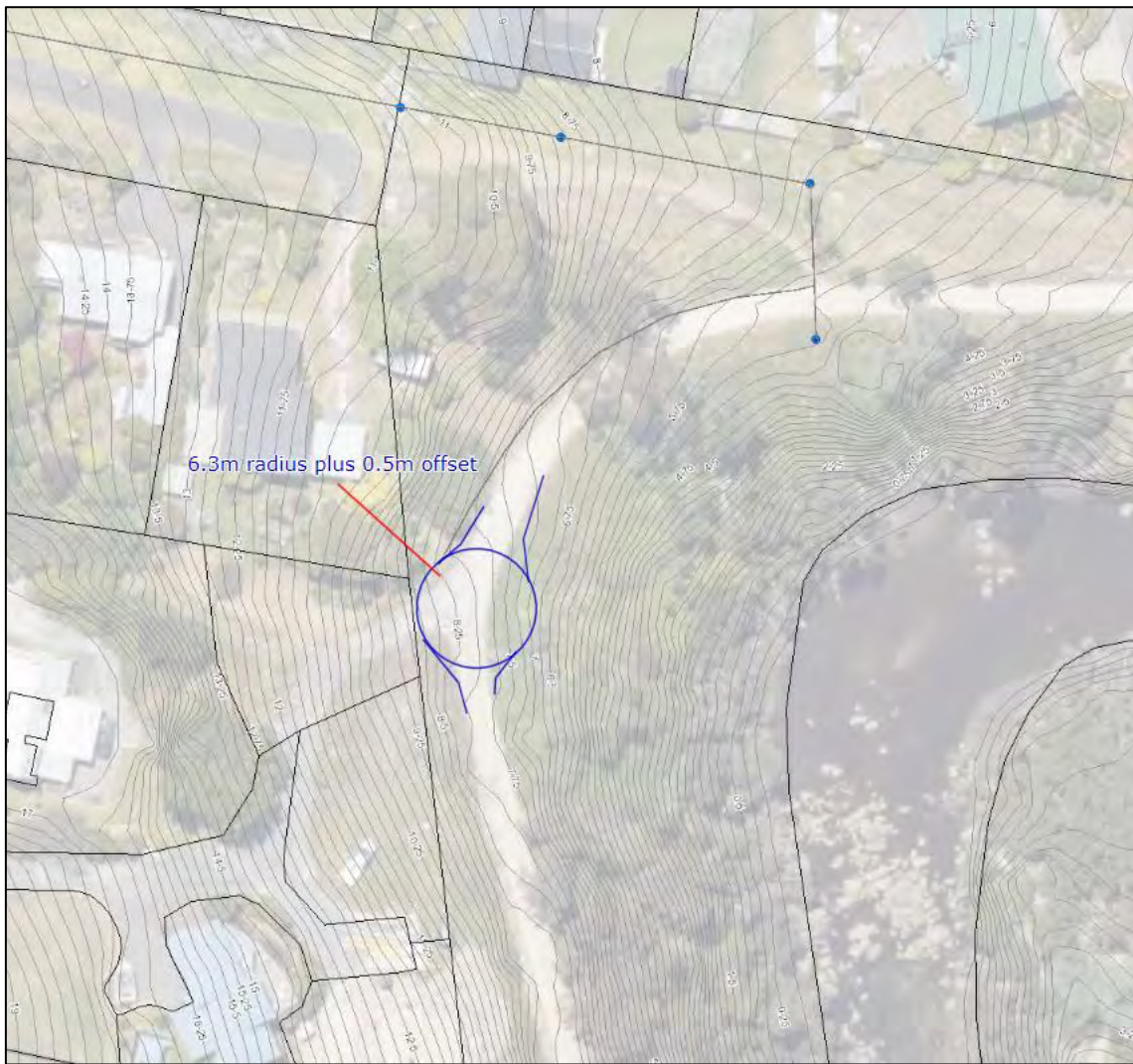
Figure 21 – Aerial imagery depicting potential 6.3 metre radius (plus 0.5 metre offset) turning area within the Esplanade and proximate to Unit 6 4 Bridview Place Bridport (adapted from www.thelist.tas.gov.au ). © State of Tasmania
